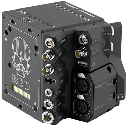
Figure: Expansor DSMC2 REDVOLT
